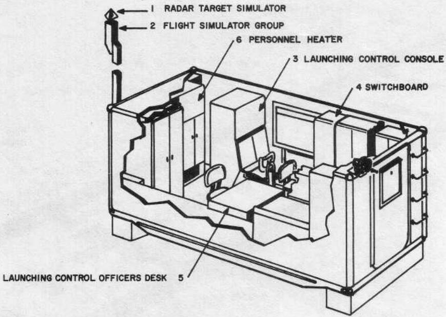
Figure 5. Launcher control trailer--permanent layout.
