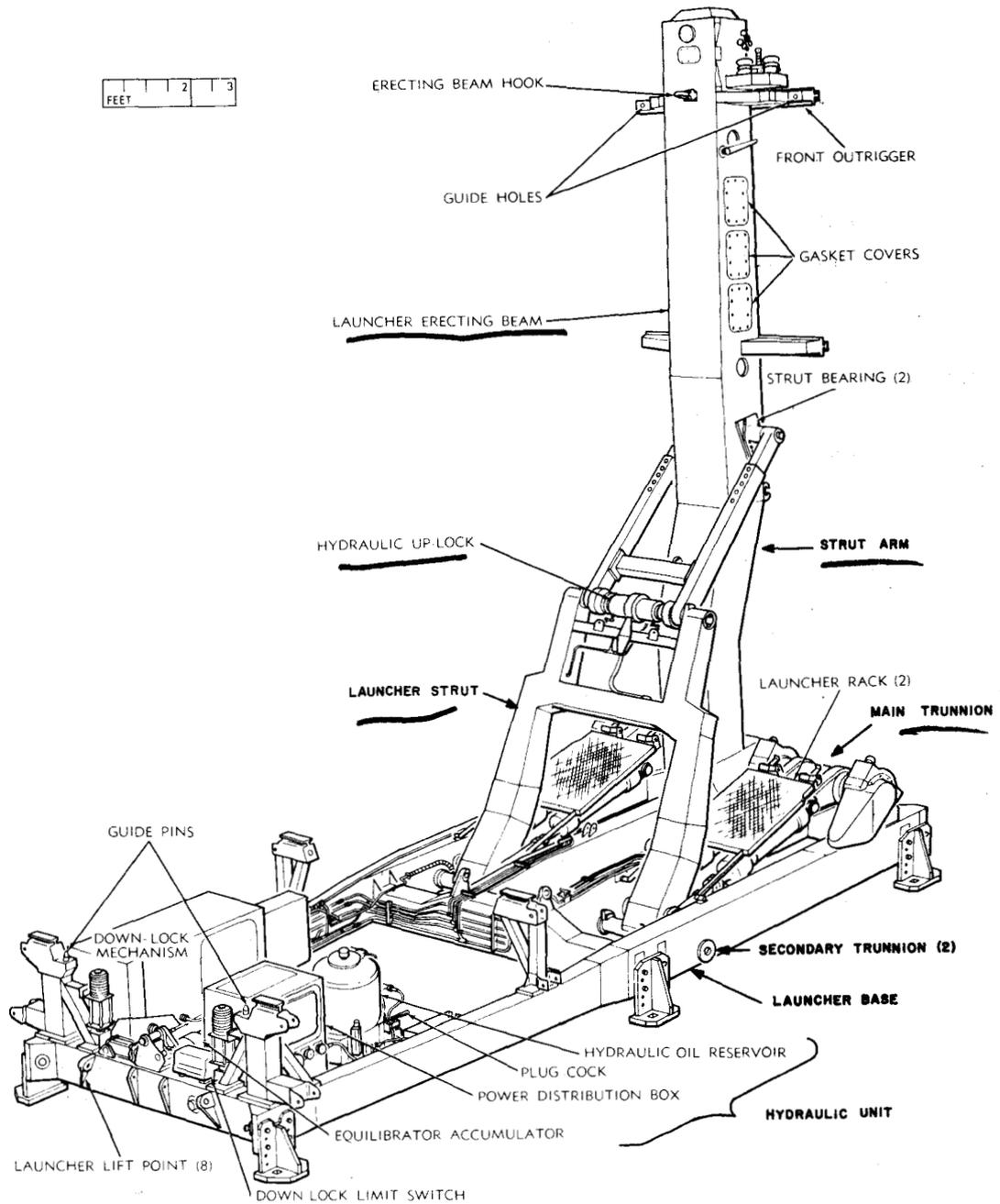
Figure 12. Monorail launcher.
