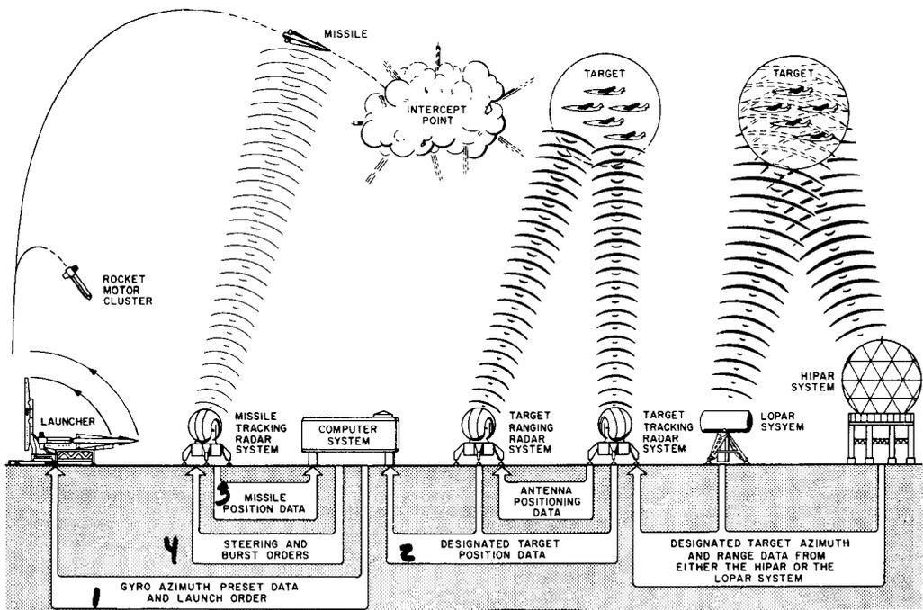
Figure 2. Surface to air mission--functional diagram.
